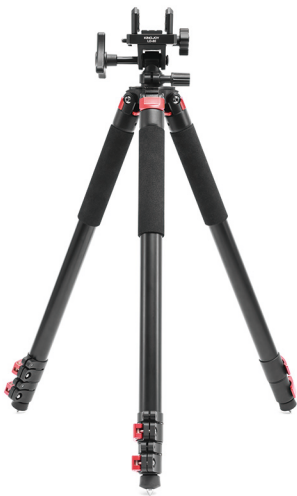
HT4007+LD-80 3-SECTION CARBON FIBER TRIPOD KIT Extended 280mm ~ 1530mm Folded 760mm Weight 3.10kg Max Load 20kg Diameter 28mm ~ 34.6mm Material Carbon Fibre Section 3
