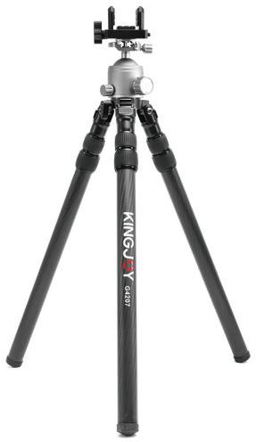
G4207+LD-80 3-SECTION CARBON FIBER TRIPOD KIT Extended 130mm ~ 1280mm Folded 625mm Weight 1.57kg Max Load 20kg Diameter 28mm ~ 34.6mm Material Carbon Fibre Section 3
