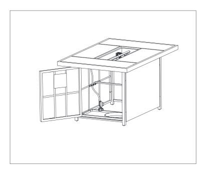
7. Turn the cylinder valve on the tank clockwise to close the propane tank. Attach the pre-assembled regulator from the table top (B) to the cylinder valve by turning the regulator coupling nut clockwise. Make sure it is fastened securely and tighten connections by hand only.
