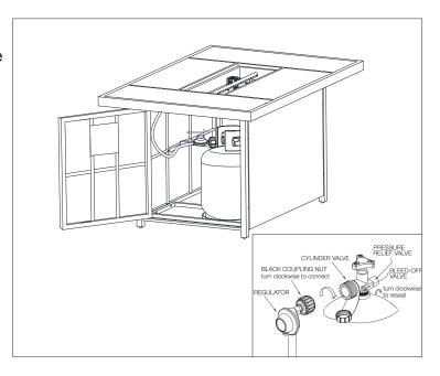
8. Place propane gas tank ( not included ) into the metal stand ( E ). Make sure the gas tank sits on the metal stand ( E ) completely. Turn the preassembled wing screw on the outer part of metal stand ( E ) clockwise to secure the propane gas tank tightly.
