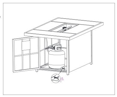
9. Remove the rubber cap on the electronic igniter (12) by unscrewing and slide battery into the battery slot. Make sure the positive side of the battery faces outwards. Screw the electronic igniter cap (12) over the battery tightly. The ignition module requires one Alkaline AA size battery (1.5V).
