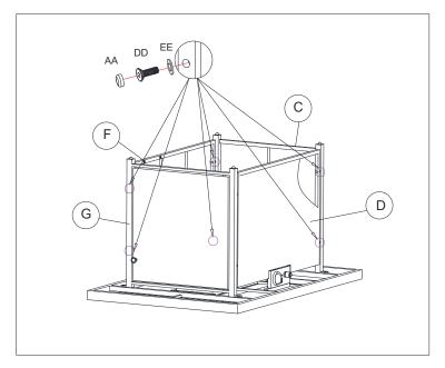
4. Attach the metal stand ( E ) to the back panel ( F ) and front panel ( D ) using four M6 x 25 screws ( CC ), four washers ( EE ) , four screw caps (AA).
