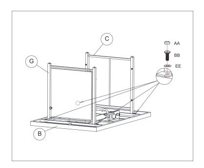
3. Attach the back panel (F) and front panel (D) to the door (G) and the side panel (C) using eight M6 x 30 screws (DD), eight washers (EE), eight screw caps (AA).
