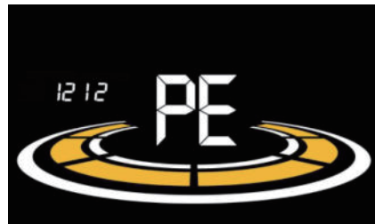
Figure 6-16 Power-on password setting interface
