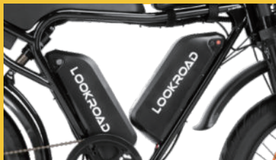
A. Recharge the battery on E-bike directly
