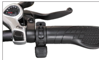
03 Throttle installation is complete.
