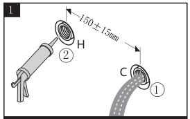
\*Turn on the water and flush the water pipe for 3minutes installation, Rinse out the sand and gravel in the water \*First seal the gap between the G1/2 water outlet and th with silicone sealant, the center distance of the 2 water must be between  $150\pm15$ mm.
