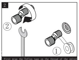
Then use a wrench to screw the two swivel elbow into the
