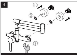
As shown in picture, install the decorative cover swivel elbow first, and then fix the faucet with a wren Note:Don't forget step 2 put the washer, avoid sand clo the faucet.
