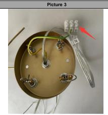
Step 2: Connect the zero line (N), fire line(L), and ground line to the terminal (F), and then connect them to the home power supply (pay attention to distinct the zero line and fire line).
