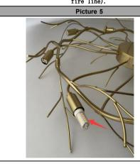
Step 4: Install light source (F) and test the light, if no problem can proceed to the next step.
