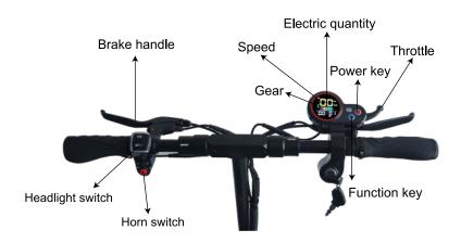
Press the accelerator lightly to speed up the electric scooter.
