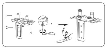
First install and fasten the clamp connector (2) under stand base (1) together, then stick anti-slip pad (9) under them.
