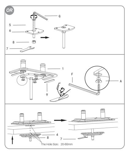
For Desk with grommet hole or hole on it, need to attach and fasten the parts together first, then install stand base through the hole on desk to fasten stand base on desk firmly.
