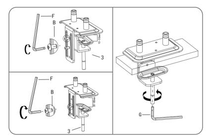
Now assembly the clamp connector with C- clamp (3) together. There are 2 positions to choose. Finally mount the stand base on desk side and fasten it.
