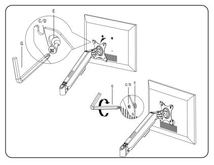
Install 2 screws (C/D) and washers (E) on the upper VESA mounting holes first. \* only half screw the screws on so that monitor can be hanged on VESA plate safely. Then hang the monitor on arm and fasten the top 2 screws, finally install the lower 2 screws on firmly.
