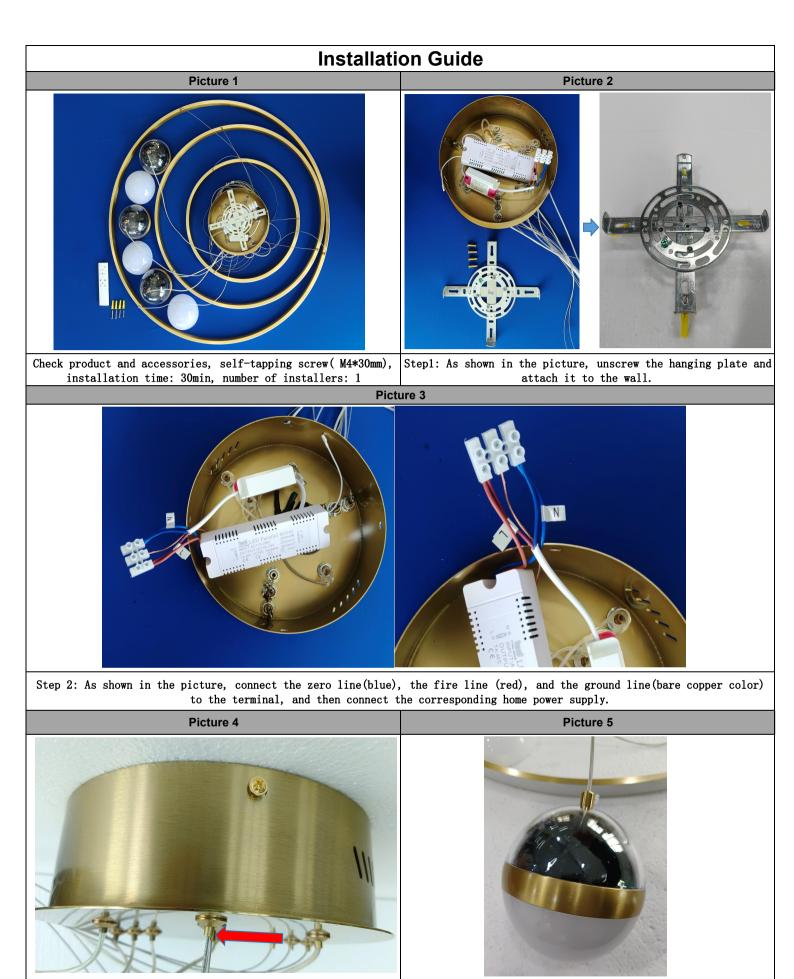
Step 3: As shown in the picture, fix the chassis to the plate, and by holding down the arrow, adjust the cable to the appropriate one.
