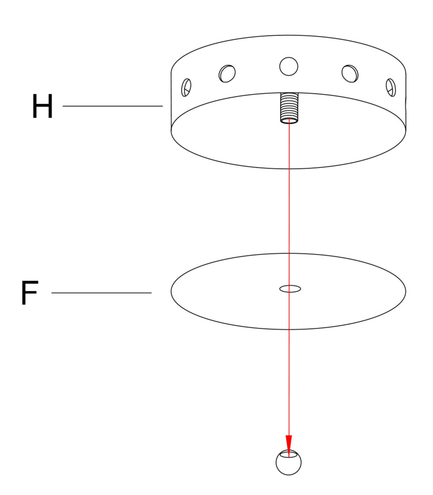
Remove the pre-installed nut first
