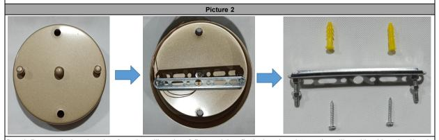
Step 1: Remove the hanging plate from the ceiling plate C first, and then fix the hanging plate on the ceiling with rubber plug H and self-tapping screws I.
