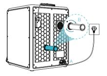
3 Load filaments. (Insert the filaments into the deepest part of Teflon tube until it cannot be moved.)
