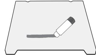
③ When the first layer of the model is not glued, it is recommended to apply glue stick evenly on the surface of the platform.
