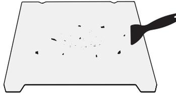
② The residue of the platform filaments can be scraped off with a blade. Be cautious of safety when using.
