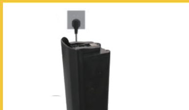
B. Remove the battery from the bike and charge it separately
