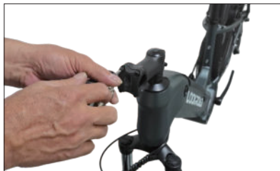
05 Remove the fixing screws (on the head tube).
