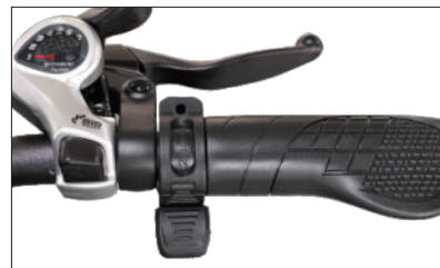
03 Throttle installation is complete.
