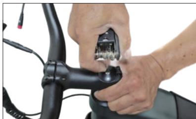
07 Secure the top screws of the head tube.
