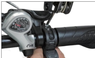
02 Loosen the throttle clamp screw, mount the throttle onto the handlebar, and tighten the screw to secure it.
