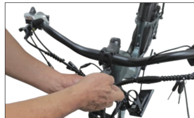
06 Install the handlebar and tighten the fixing screws.
