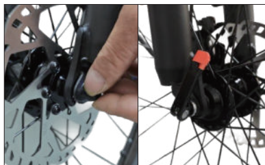
05 Mount the front wheel onto the front fork, attach the fixing screws, and lock the front wheel axle securely.
