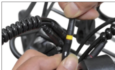
01 Connect the throttle cable correctly (align the connectors to avoid reverse insertion).
