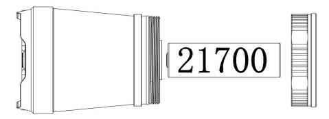
Unscrew the tail cap to insert one 21700 battery with the anode side (+) towards the head, then screw the tailcap back on.
