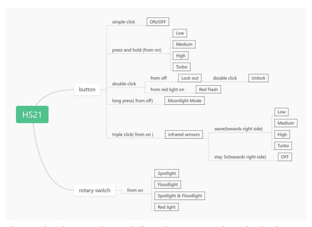
The HS21 has three switches, and all switches operate independently. The rotary switch is used to switch between different modes, while button and infrared switch are used to select different brightness levels.
