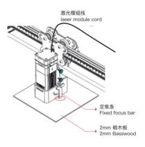
Please place the multi-level fixed focus bar between the laser module and the processed material. Follow the tips and make the bottom of the laser module contact with the corresponding surface of the multi-level fixed focus bar. Finally lock it with two hand screws on the right. For example, if you engrave or cut a 2mm basswood or other material:
